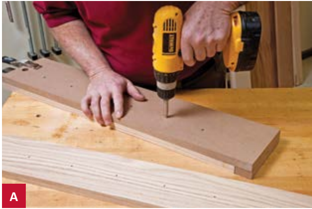
Figure 2: Front Rail Drilling Jig and Back Rail Template
