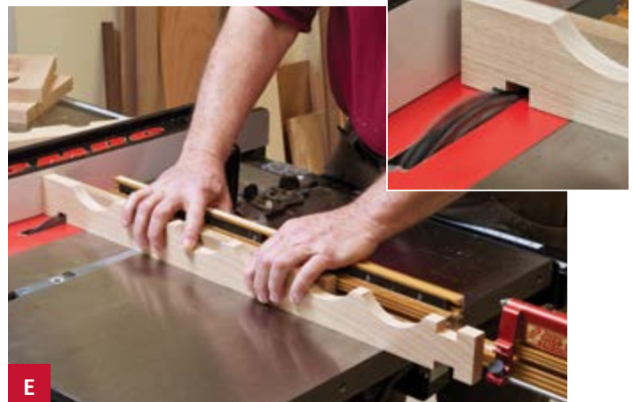
E Working between the miter gauge stop and saw fence, make the dado cuts in two passes.
