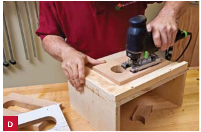
D Jigsaw rough openings in the end blanks and MDF piece, using a stand that has a fence and blade-clearance opening in its top.
