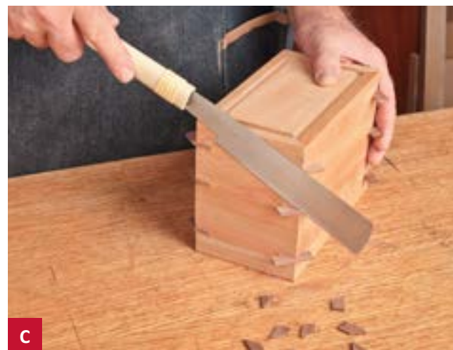
Cut the protruding spline ends flush with a fine-tooth flush-cut handsaw.
