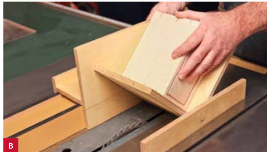
With the fence adjusted, use the box splining jig to make the first spline cuts in all four corners before moving to the next set of cuts.
