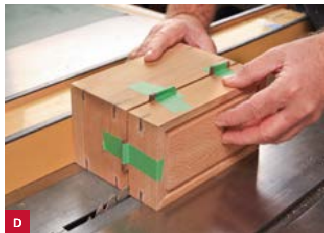
To ensure accuracy and safety, tape spacers in the kerfs as you make the final two cuts around the perimeter of the box.
