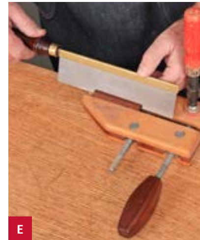
With the lid lift clamped firmly as shown, angle a stiff fine-toothed saw such as a backsaw to cut the card-holding kerf.
