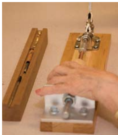
A STANDARD PEN PRESS finishes the job. Note the "story board" used to organize pen parts for assembly.
