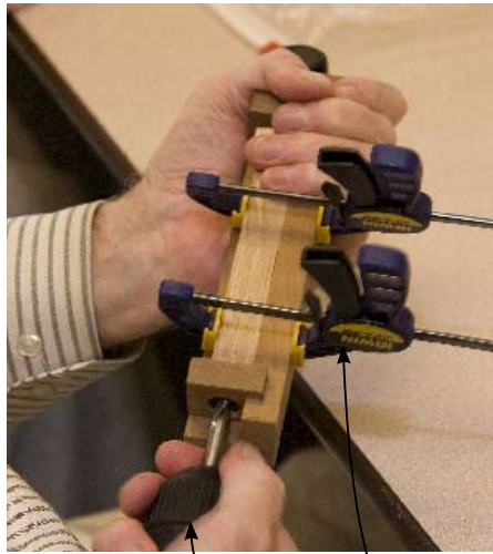
mini-clamps to secure assembly (Woodcraft clamp #130925)
