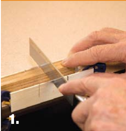
A MINI MITER BOX and fine-toothed saw are used to cut common pen blanks to size.
