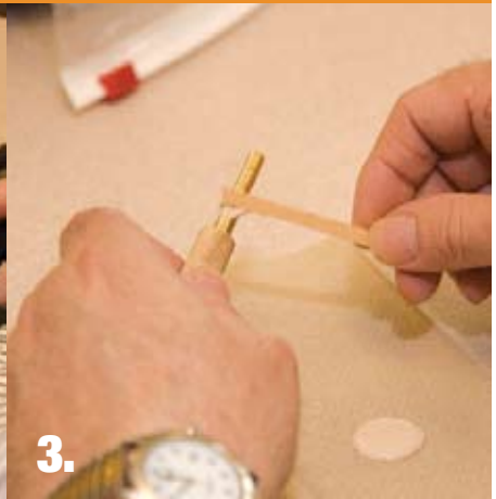
SANDED BRASS BUSHING are glued into the blanks with regular wood glue, which has plenty of strength for the task and is safe for residents.
