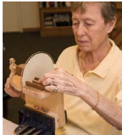
SQUARING THE ENDS and removing excess glue can be done without power or a pen mill, thanks to this hand-cranked disc sander Larry Beckwith devised. Pat Huyvaert holds a pen part steady in the cradle while sanding.
