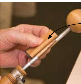
Final sanding using 600-grit sandpaper and contour sanding block (Woodcraft #14958)
