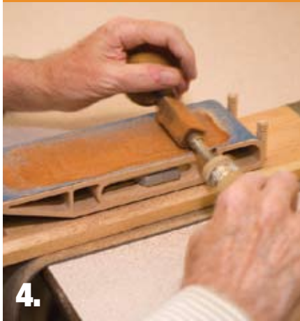
A SANDING BLOCK CRADLE on a non-slip pad facilitates vigorous sanding. Two sets of bushings are used to guide the process.
