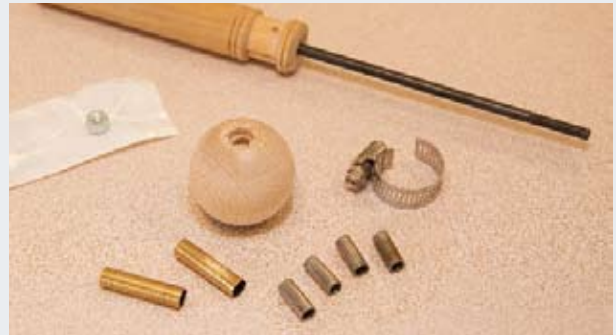
START GATHERING THE SUPPLIES you will need to make specialized tools for making pens by hand. Items include a keyless chuck, 7-mm drill bit, hose clamp, and bushings in two sizes.
