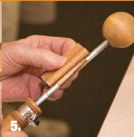
THE OUTER BUSHINGS are removed, and the Penwright moves to hand sanding with a contoured rubber block.
