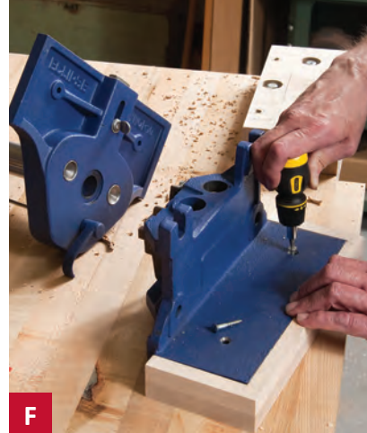
F Attach the rear cheek with #10 flathead woodscrews after countersinking the holes in the jaw.
