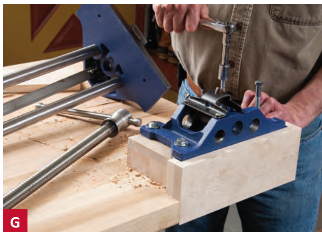
G Snug the rear jaw assembly firmly in place while tightening the lag screws.
