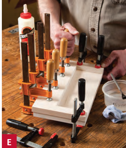
E Glue the U-shaped cheek filler to a piece of \frac{3}{4} "-thick stock to make the rough-sized rear cheek.
